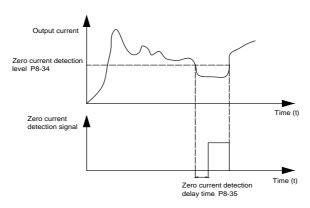
Figure 6-20 Zero-current detection diagram
