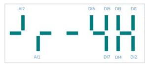
Each segment of LED indicates one digital input terminal.
