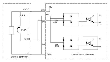
Figure 3-18 PNP type wiring
