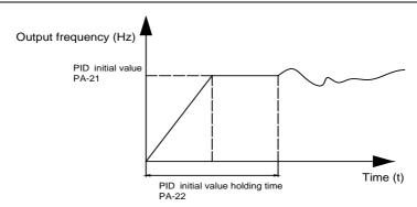
Figure 6-26 PID initial value function diagram
