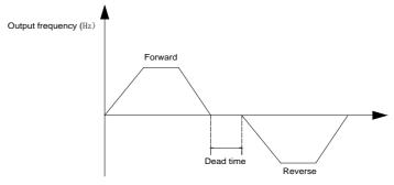
Figure 6-14 FWD/REV dead time diagram
