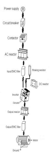
Figure 3-2 Diagram of the connection to peripheral devices
