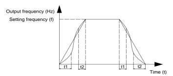
Figure 6-10 S curve ACC/DEC diagram
