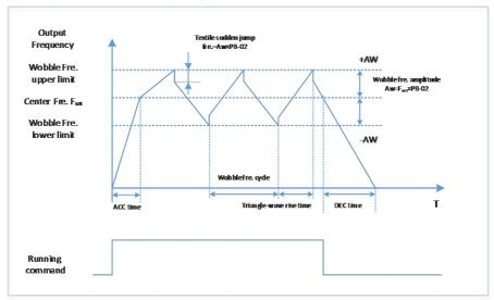
Figure 6-27 Wobble frequency operation diagram
