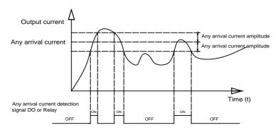
Figure 6-22 Any arrival current detection diagram
