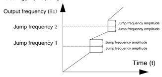
Figure 6-17 Jump frequency during ACC/DEC diagram
