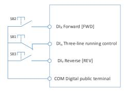
Figure 6-7 Three-line Running Mode 1
