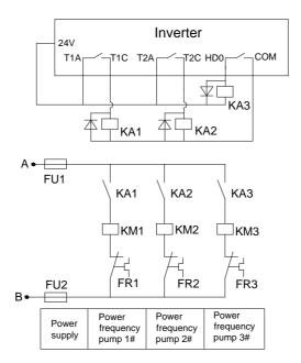
Figure 6-32 Constant pressure water supply electrical schematic diagram
