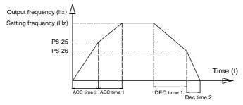
Figure 6-18 ACC/DEC time switching diagram
