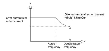
Figure 6-33 Double-speed over-current stall action diagram
