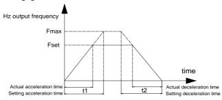
Figure 6-1 ACC/DEC time diagram
