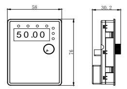
Keypad dimension of 1AC/3AC 220V 0.4~1.5kW inverters
