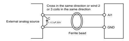
Figure 3-16 Connection of analog Input
