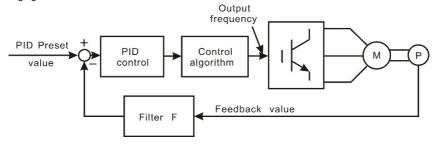
Figure 6-24 PID control diagram
