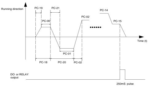
Figure 6-29 Simple PLC diagram
