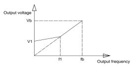
Figure 6-3 Manual torque boost diagram
