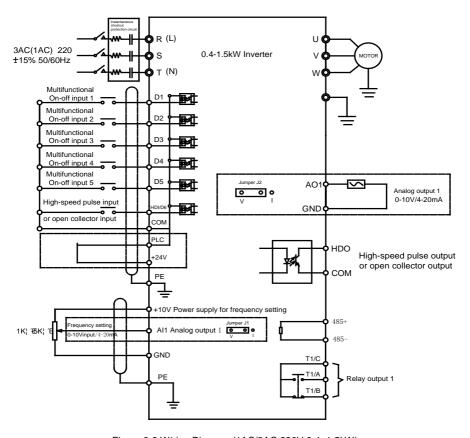
Figure 3-3 Wiring Diagram (1AC/3AC 220V 0.4~1.5kW)
