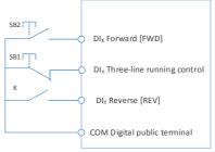
Figure 6-8 Three-line Running Mode 2
