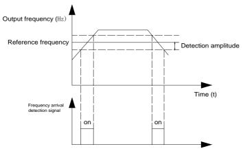
Figure 6-16 Frequency arrival detection diagram
