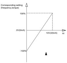
Figure 6-9 Corresponding Relationship between Analog Reference and Setting
