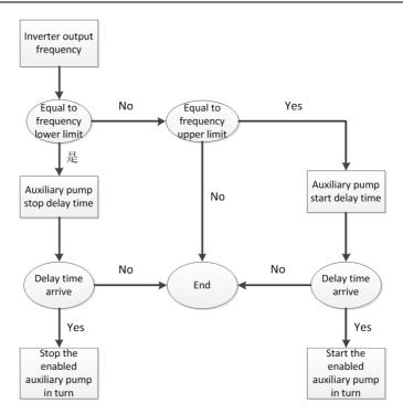
Figure 6-30 Constant pressure water supply logic diagram
