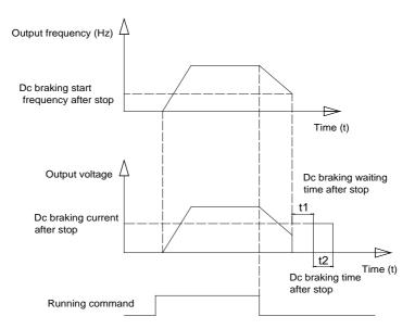
Figure 6-12 DC braking diagram
