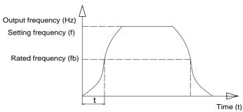
Figure 6-11 S-curve ACC/DEC A diagram
