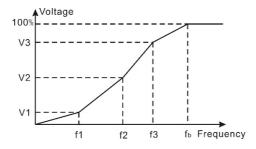
Figure 6-4 V/F curve setting diagram
