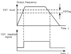
Figure 6-15 FDT Level and lag diagram
