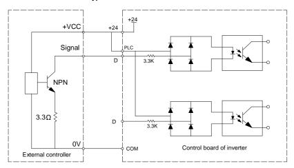
Figure 3-17 NPN type wiring
