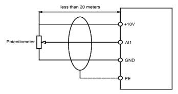
Figure 3-15 Connection of analog input
