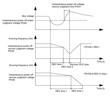
Figure 6-23 Instantaneous stop action diagrams
