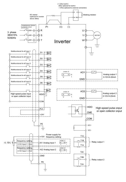
Figure 3-4 Wiring Diagram (>1.5kW)
