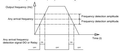
Figure 6-19 Any arrival frequency detection diagram
