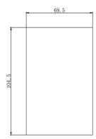
65\*100mm hole dimension of keypad bracket
