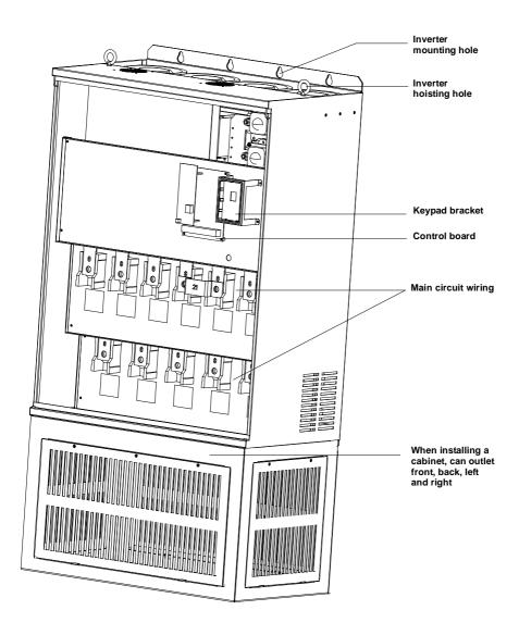
Figure 2-3 Parts of inverter
